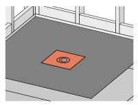
Avoid sloping mortar onto membrane that is adhered to the ClearPath Drain Plate.
