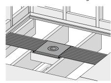
9 Screw down TI-ProBoard® starting with boards centered on the drain plate. Use two of the screws to fasten TI-ProBoard to drain plate on each butt edge. Work from the center out to each edge. Placing one screw on each of the marked channels on each joist.
