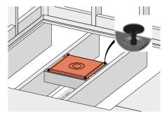
6 The ends of TI-ProBoard must be fully supported by at least one half of a joist if not available, blocking must be installed.
