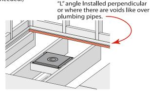
8 TI-ProBoard must be installed perpendicular to the joist. Starting with the pieces that butt into the drain plate, measure, cut and dry fit the TI-ProBoard to the shower floor opening. TI-ProBoard® must land on at least three joists or end blocking. A wet saw is recommended for cutting TI-ProBoard.
